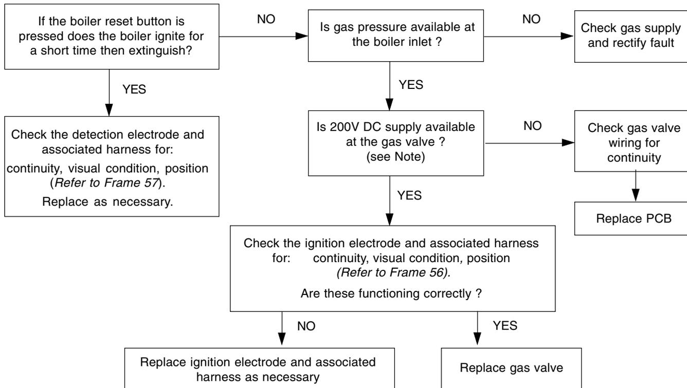
**Note.** Due to the wave form of the rectified voltage, the reading will vary depending on the type of meter used to measure the value (some may measure the possible peak voltage of 339V). In general terms a reading greater than 150V indicates that the correct voltage is supplied to the gas valve.
