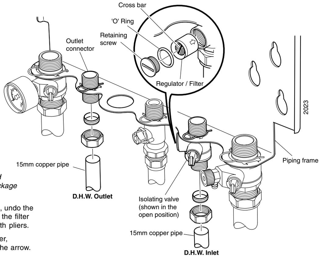
**Note.** The DHW inlet isolating valve incorporates a flow regulator / filter. It should be inspected to ensure no blockage is evident.
