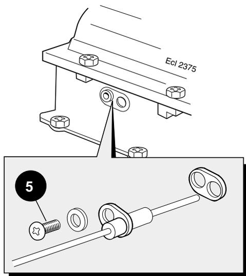
5. Remove the screw holding the flame detection electrode to the combustion chamber.
