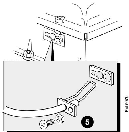
5. Remove the screw holding the ignition electrode to the combustion chamber.
