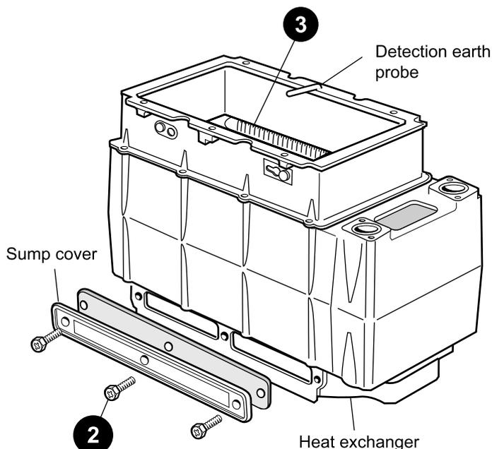
**Note.** Take care not to disturb the detection earth probe at the rear of the combustion chamber.
